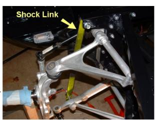
**Sidebar:** The heavier torsion bars that I've selected are just a bit stiffer than stock. Using the stock shock link with these heavier bars would make the car ride higher than stock. Plus, since I wish to run a lower-than-stock ride height, I will certainly need to use a shock link that is shorter than 17-13/16 inches. But how much shorter? That's the \$10,000 question (and why I'm installing the adjustable reaction plate)!
