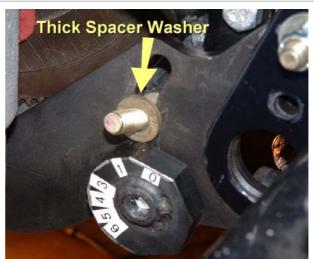
Place a small amount of grease on the shoulder of the support ear where it passes through the reaction plate. Place the shoulder of the support ear through the subframe plate and reaction plate. Feed the slot bolt through the support ear. Place a washer, lock washer and nut on the slot bolt.
