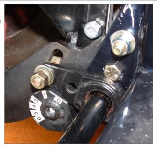
Now turn your attention to the front of the torsion bar. Slide the bar forward and align the front end of the bar with the back of the splined hole in the lower control arm. Chances are, the bar will not want to slide into the lower control arm because the splines are not lined up. This is because there are 25 splines on the rear of the torsion bar, and only 24 on the front.
